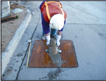
The slump flow test is done on a flat surface using a standard slump cone. After filling, the cone is lifted and the diameter of the resulting pat is measured.
