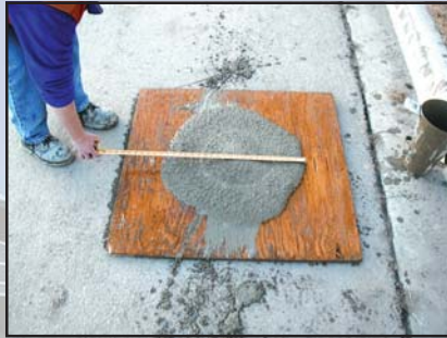
The slump flow test is done on a flat surface using a standard slump cone. After filling, the cone is lifted and the diameter of the resulting pat is measured.
