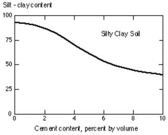
Fig. 4. Reduction in Silt-Clay Content Due to Cement Modification
