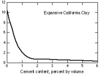
Fig. 2. Expansion versus Cement Content, Highly Expansive Clay
