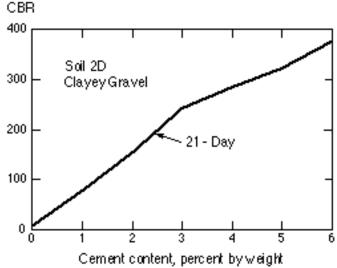
Fig. 7. California Bearing Ratio versus Cement Content
