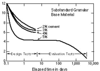
Fig. 6. Reduction in Plasticity Index Due to Cement Content and Time
