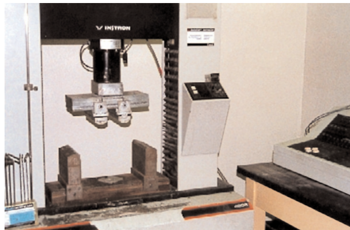
Figure 2.12. Flexural strength testing equipment. (IMG15529)
