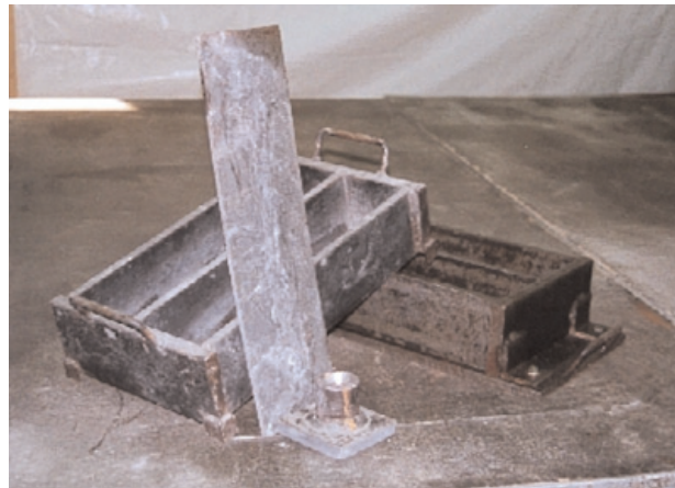
Figure 2.7. Molds used for consolidation of beams. (IMG15524)
