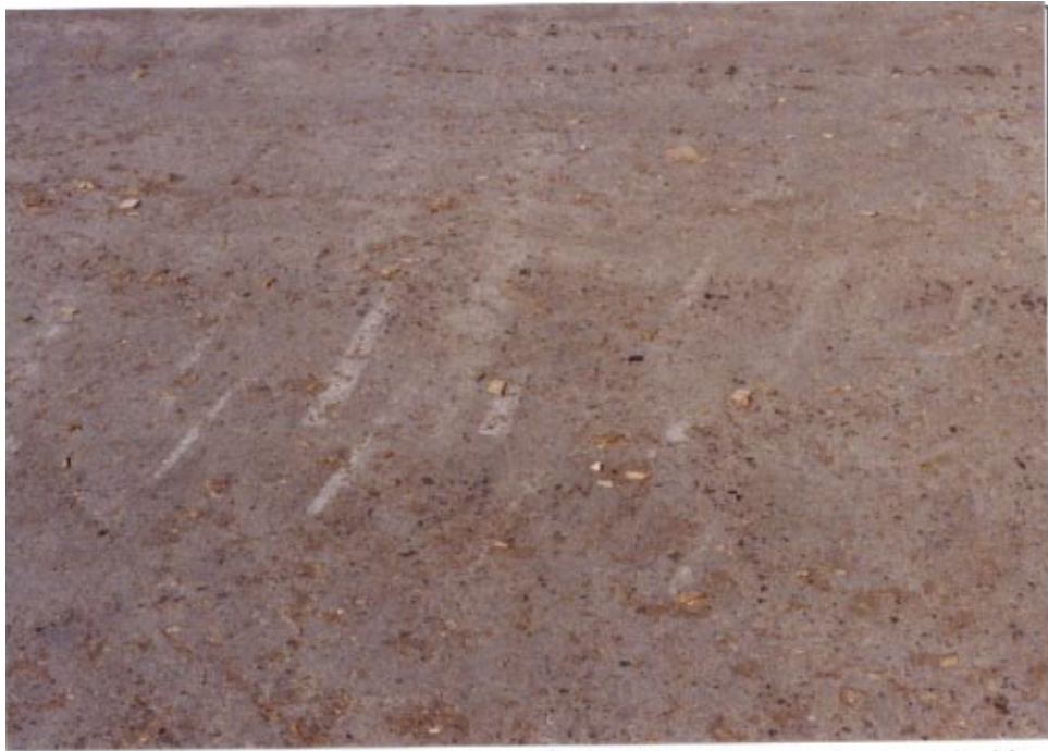
Figure 37 Bulldozer lugged tracks only scuff the surface of the RCC chip storage pile base.
