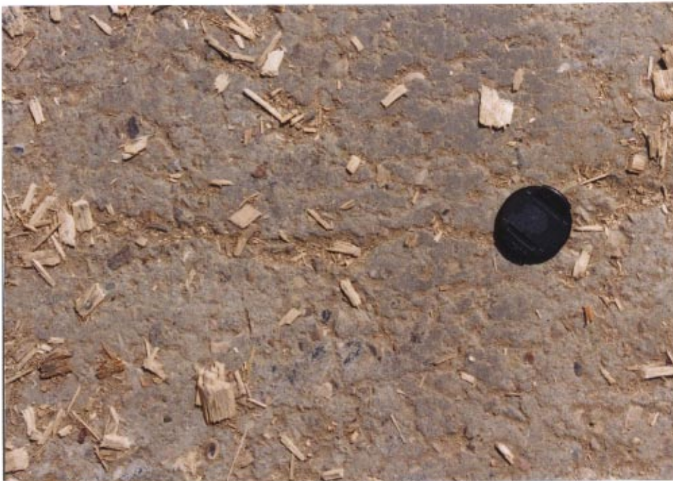
Figure 6 Wood fibre in the shrinkage crack. Alberta Pacific Forest Industries, Athabaska, AB. Built in 1992.
