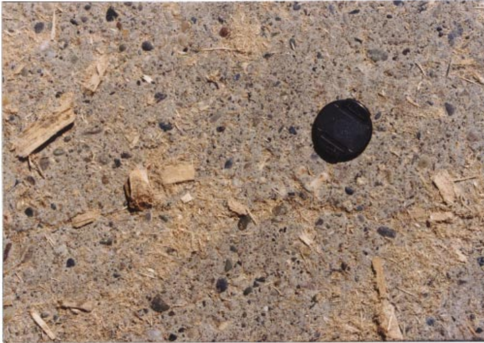
Figure 32 Shrinkage cracks remain tight. Debris from the wood chips fills any space.
