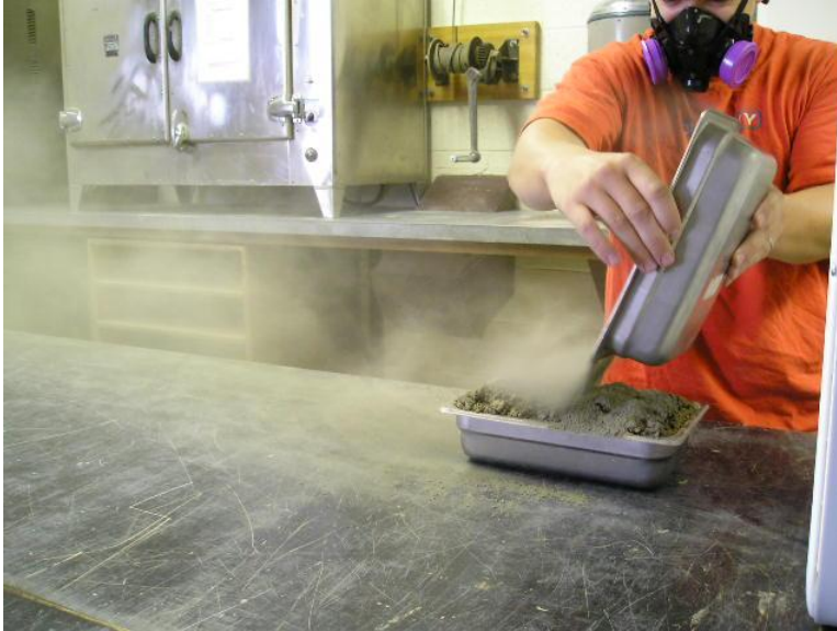
Figure 2. Cement powder dispersion during blow test.
