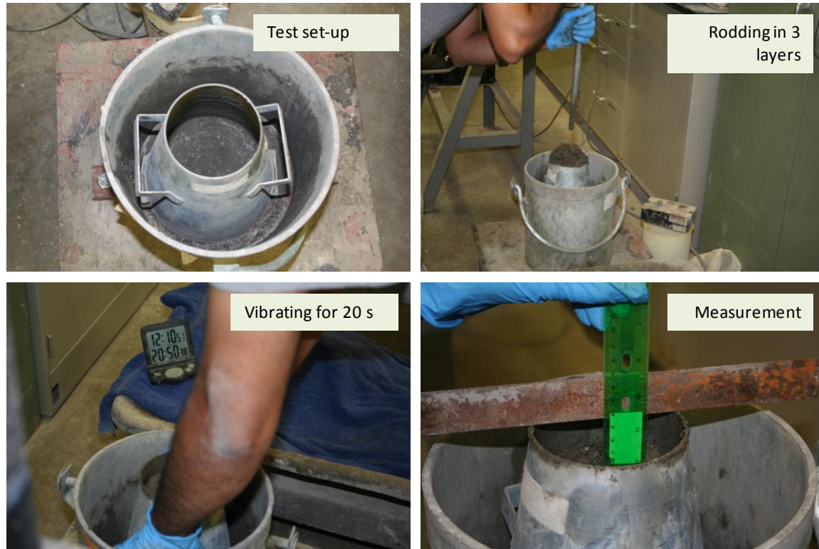
Figure 3-1 Test procedure for measuring consistency: CSV
