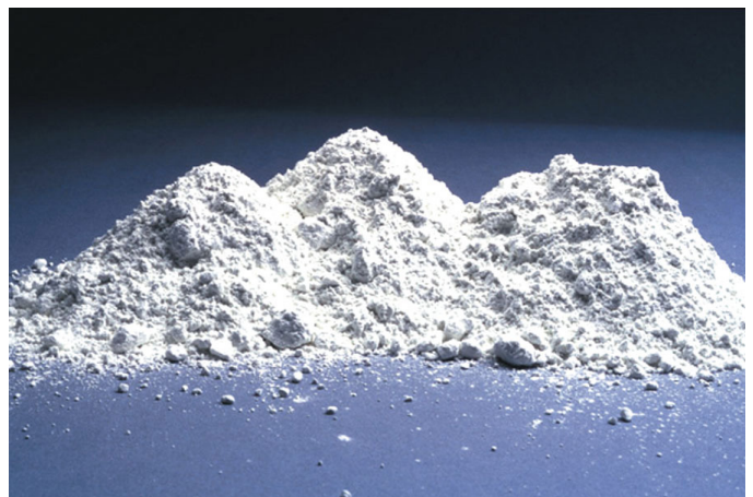
Figure 2. White cement is subject to exacting quality control procedures that minimize color variation during manufacturing.
