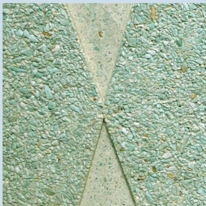
Figure 6. Lightly sandblasting over a pattern created using rubber inserts results in a surface with color, texture, and relief. A white cement matrix anchors the green aggregate (cordierite), whose color predominates.
